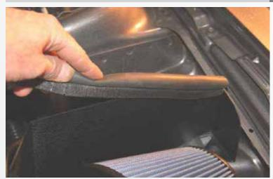
Install the supplied sponge seal to the top of the air filter shield and trim off any excess
