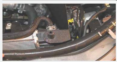
Install the BBK air filter shield into place and position over the radiator mount peg with the rubber grommets seating into their holes in the inner fender. Install the stock bolt back into the small tab on the shield and tighten the bolt. Re-install the upper radiator mount and tighten the bolts.
