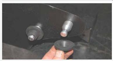
Assemble the 2 aluminum pins to the bottom of the BBK air filter shield using the supplied  $\frac{1}{4}$ -20x  $\frac{1}{2}$ " Phillips screws. Install the stock rubber grommets onto the pins.
