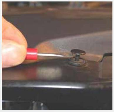
Remove the plastic radiator cover by prying up the center of the plastic pin heads at the slots cut on each side. Pull the pins out to remove. Lift cover and set aside.
