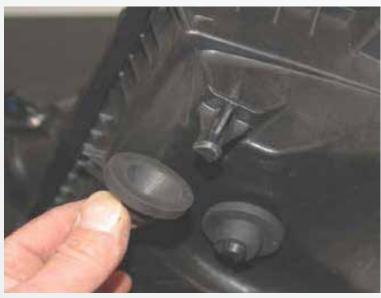
Remove the bolt on the right side of the stock air box that mounts it to the inner fender. Detach the air box from the lower inlet tube on the side of the radiator as you lift the box out to remove. Detach the Mass Air Sensor wire harness from the side of the air box by slightly pulling on the harness at each barbed mounting pin. Remove the 2 rubber grommets from the bottom of the air box.
