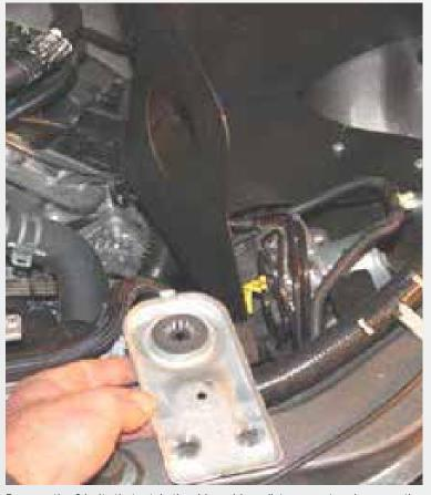
Remove the 2 bolts that retain the driver side radiator mount and remove the mount.
